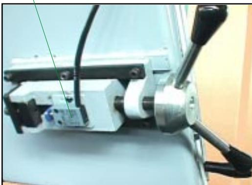
When replacing a blade, ensure that the belts are 0,9 mm thick as the guiding blade pads have been adjusted to this size. If using different size toothed belts, it will be necessary to proceed with a new registration as follows:
