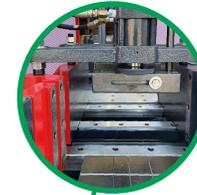
HYDRAULIC CLAMPING (BEAM CLAMP OPTIONAL)
