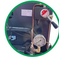
HYDRAULIC BELT TENSIONING DEVICE
