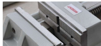
With prism insert clamping jaws
