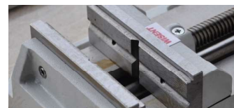
With prism insert clamping jaws
