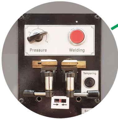
Cutting, welding and grinding device for bandsaw blade
