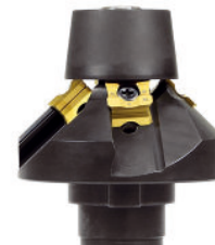
fig. 45°-radius-milling head with 4 cutting edges and guide roller, equipped with 4 mm-radius-indexable inserts of type R-K
