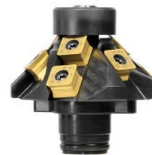
fig. 45°-bevel-milling head with 3x3 cutting edges and guide roller, equipped with 9 bevel-indexable inserts of type K
